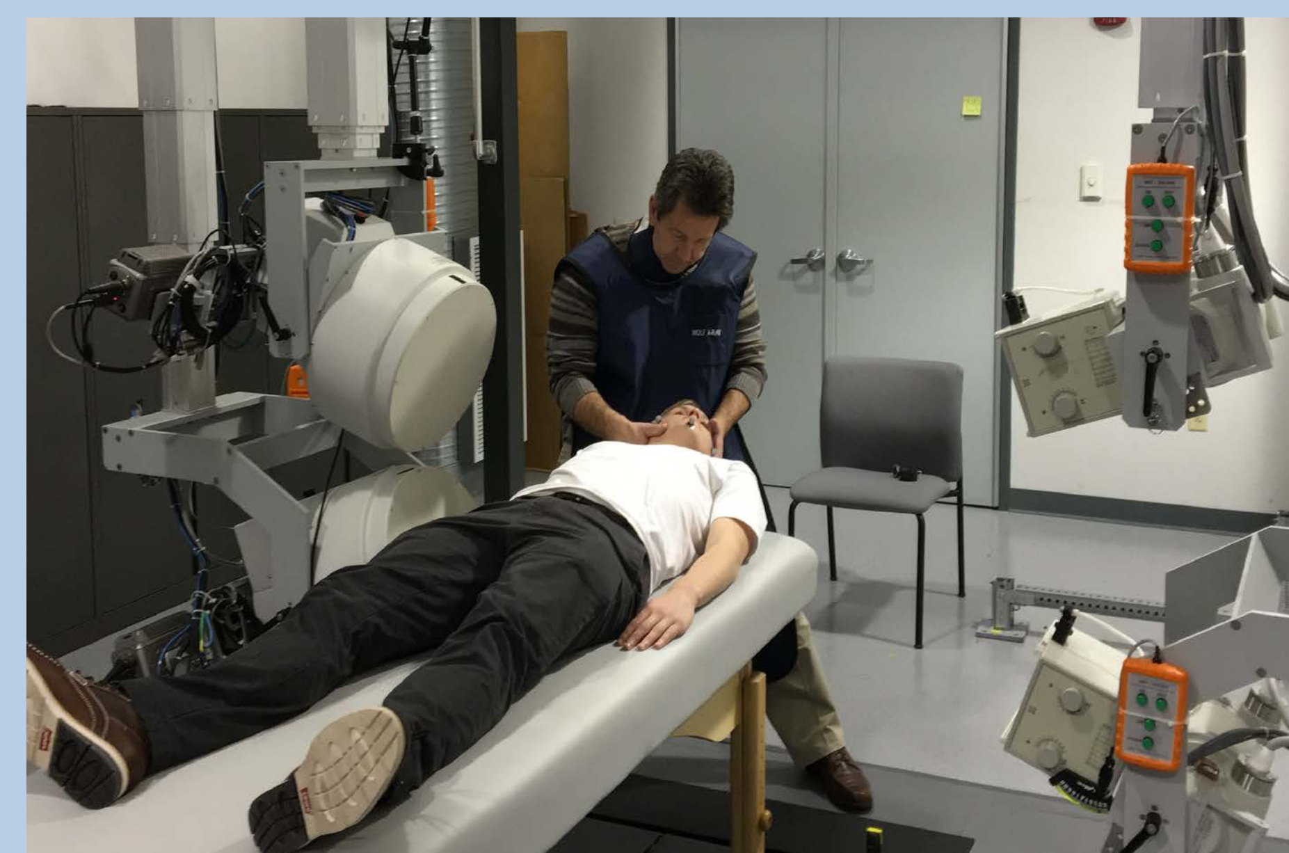
Figure 1. The biplane imaging system configured to collect dynamic biplane radiographs during HVLA manipulation. The X-ray sources are to the right, and image intensifiers and high-speed cameras to the left, providing sagittal-oblique views of the spine without occlusion from the clinician.
